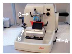
The knife holder base clamp A, the lateral displacement clamp B, and the x-y orientation clamp C should be firmly locked before trimming your block. Failure to do so may result in damage to both block and blade.
