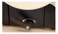
The handwheel brake of the Leica RM2235 is shown here in the locked position. The brake can be activated with the handwheel in any position. Either the handwheel lock or the handwheel brake can be used to immobilize the microtome.
