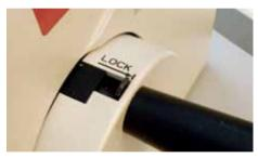
The handwheel lock is shown here with the handwheel in the 12 o'clock position and the lock engaged. This lock will only engage in this position at the top of the cutting stroke.
