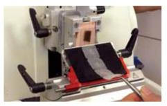
This ribbon has been cut with a slow and steady stroke from a well processed, thoroughly chilled block. The sections show very little compression even before flotation.
