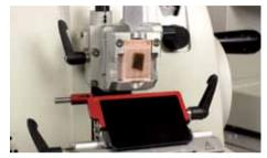
The red safety guard on the Leica RM2235 Microtome has been flipped up into place in this illustration. It completely covers the cutting edge of the blade.
