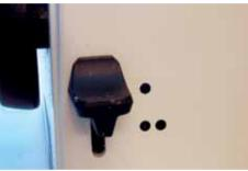
The mechanical trimming device should be used carefully when roughing, particularly the lower (..) setting that produces an advance of 30 µm when activated.
